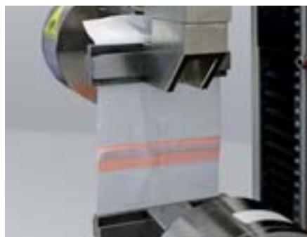
In seam strength tests performed in accordance with EN ISO 13935-2, mechanical pulling force is applied to the material to determine the level of force required to rip the seam.
