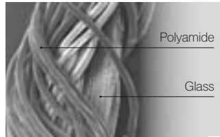
Solid construction. Core – shell – thread.
