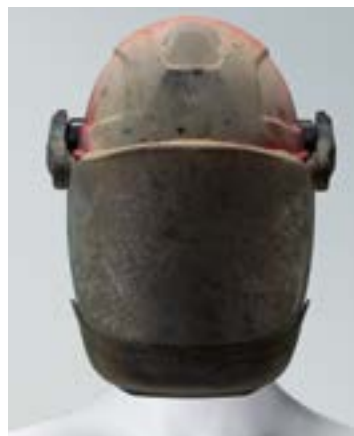
According to 7 kA short circuit electric arc
