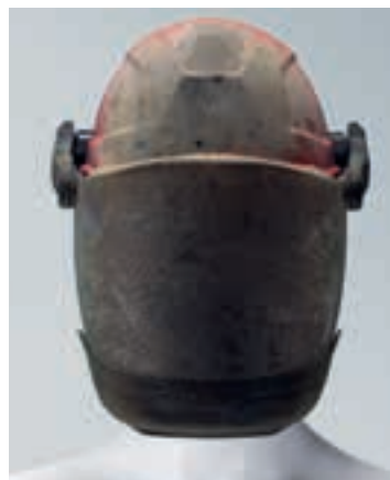
According to 7 kA short circuit electric arc
