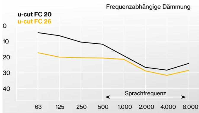
**uvex high-fit u-cut FC 20** (schwarzes Filterelement)
