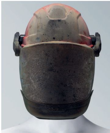
According to 7 kA short circuit electric arc
