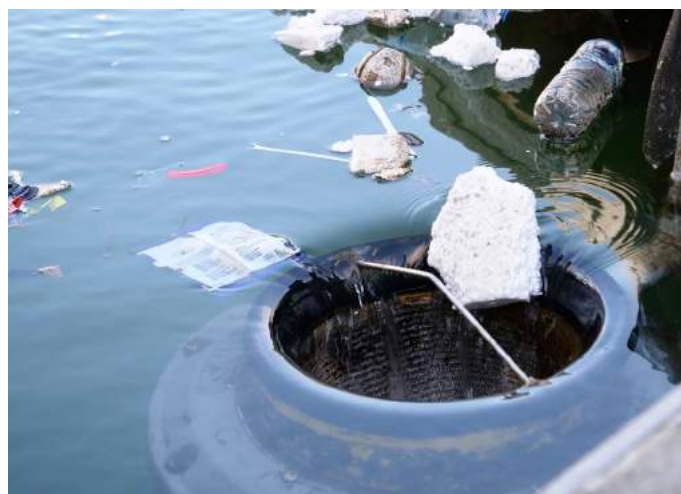
Figure 2: Marine litter captured using the Seabin smart technology in Sydney Harbour.
