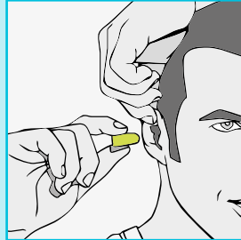
Put your arm over your head and move the ear slightly upwards to straighten your auditory canal. This achieves a better fit.
