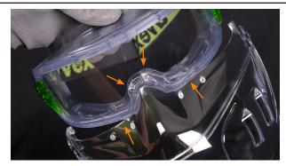
Align the goggle and shield so that the two small clips at the nose bridge clip over the rubber frame that runs along the bottom edge of the goggle.
