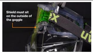
Once clipped together the face shield frame should sit on the outside of the goggle as pictured. Only the nose and side clips are inserted in to the frame.
