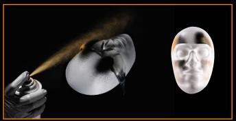
When sprayed directly with a reagent, the X-tended eye shield does not let a single droplet through – whether sprayed from the front (as per the standard), from above or laterally.
