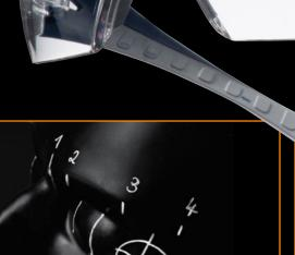
The distance between the forehead and spectacles has been measured at four different points, confirming a snug and secure fit.
