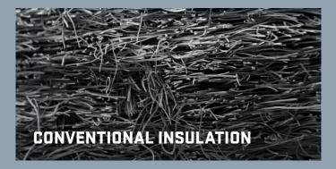
more solid fibres increase weight | the flat 2D layered structure prevents air from entering | loss of insulating capacity when compressed | fibres bon together limiting flexibility
