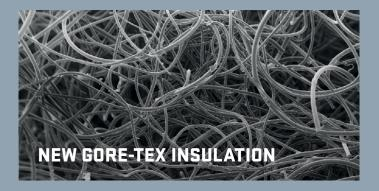
15% lighter | hollow and fewer fibres reduce weight | the 3D structure makes it possible to store more air for increased insulation | spiral effect ensures flexibility and comfort
