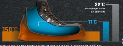
The norm states, the temperature inside the footwear must not increase in excess of 22°C for the duration of the 30 min test. The MACASPHALT internal temperature only sees a rise of 11°C, ensuring it is well within the EN 20345 HI certification.
