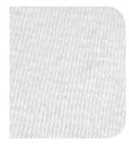
However, because it is an open-weave knit material, Kevlar® is susceptible to small punctures through the knit penetrating the skin. This has resulted in severe injury with punctures through a glove, tearing the skin. Ultraviolet exposure and temperature extremes also degrade the fibers, resulting in declining performance over time.
