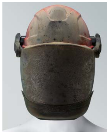
According to 7 kA short circuit electric arc
