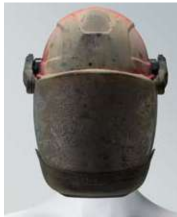
According to 7 kA short circuit electric arc
