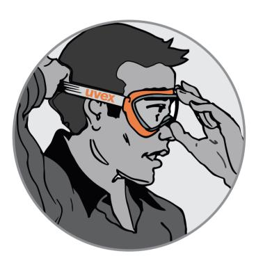
Step 3 Adjust head band to head size
