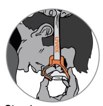
Step 1 Lean slightly forward facing down and pull head band over the top of the head
