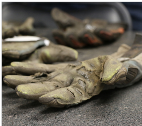
Unexpected wear on the palm during glove trials called for a visit to the mines.
