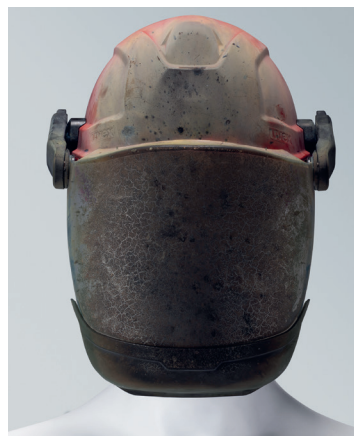
According to 7 kA short circuit electric arc
